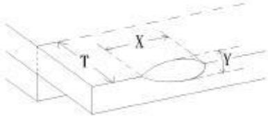
$\Phi = (x+y)/2 > 2.5 \text{ mm}$<br>Reject                                                                                                                |
